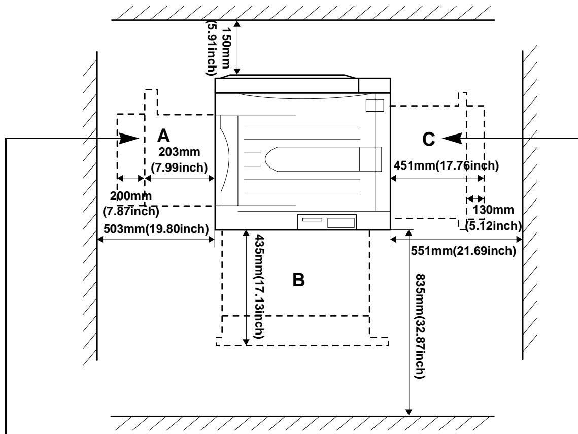
**A:** Maximum extension of the fuser unit when pulled out.
