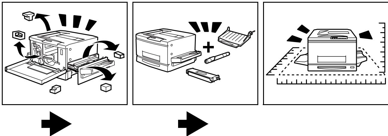
Removing the protective materials from around the printer (see page 8 to 17)
