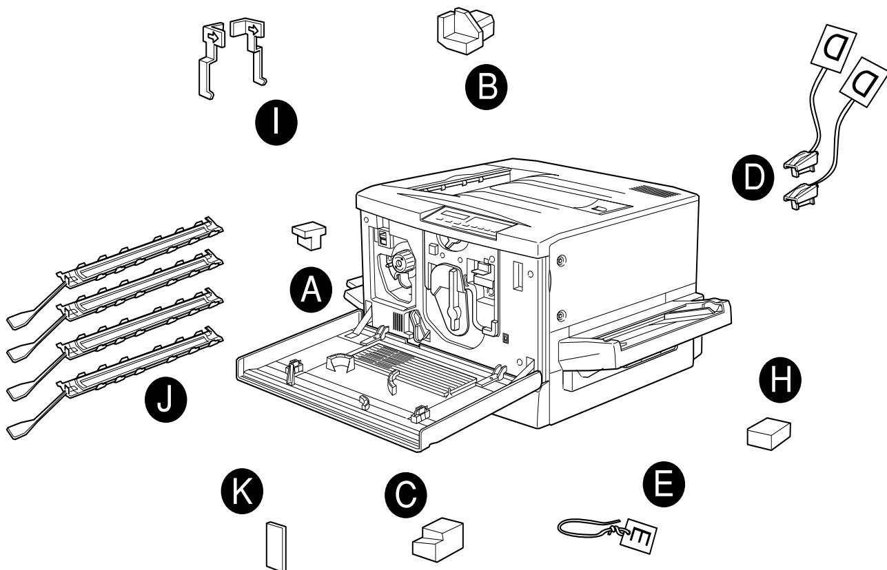
**!** Caution: In order to avoid causing damage to the printer, remove all protective materials as shown above.
